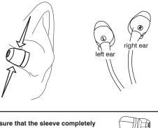
Make sure that the sleeve completely covers the earphone nozzle. If any part of the nozzle is exposed, the sleeve is not properly installed.
